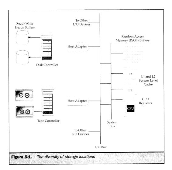
cache-buffers that are highly volatile. These components are used for only temporary locations and are staged in physical locations in increasing proximity to the CPU. The nearest component to the CPU is the fastest, and thus it is more volatile with the data it transports.
